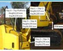
Details Rises on right hand side (i.e. maintenance) access system vary between 120 mm to 350 mm. Goings on right hand side (i.e. maintenance) access system vary between 175 mm to 300 mm.
