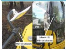
**Details** Mirror mounts and mirrors protrude from handrails on cabin access system and mirror mounts from handrails on right hand side (i.e. maintenance) access system.
