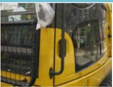
**Details** 10 mm mounting bolts on handrails for cabin entry.
