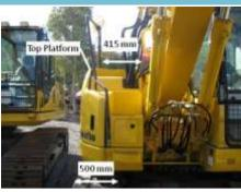
**Details** Top platform landing width on right hand side (i.e. maintenance) access system is 415 mm compared to the maximum stairways width of 500 mm.
