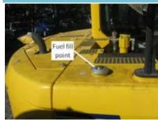
**Details** Fuel fill point partially obstruct walkways on the top platform of the machine.
