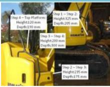
Details Step 1 dimensions on right hand side (i.e. maintenance) access system is 200 mm by 325 mm. Step 2 dimensions on right hand side (i.e. maintenance) access system is 175 mm by 235 mm. Step 3 dimensions on right hand side (i.e. maintenance) access system is 300 mm by 200 mm. Step 4 dimensions on right hand side (i.e. maintenance) access system is 190 mm by 120 mm.
