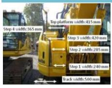
**Details** Step 1 tread width on right hand side (i.e. maintenance) access system is 240 mm compared to the maximum stairways width of 500 mm.
