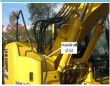
**Details** The diameter of the handrail on right hand (i.e. maintenance) access system is 32 mm.
