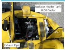
**Details** Exhaust pipe, radiator header tank and oil cooler may become hot during and following operation.
