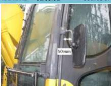
**Details** 50mm clearance on cabin access handrail due to mirror mount and mirror.
