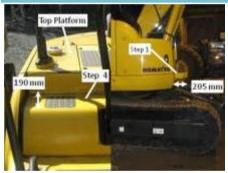
Details Depth of step 1 on right hand side (i.e. maintenance) access system is 205 mm. Depth of step 4 on right hand side (i.e. maintenance) access system is 190 mm.
