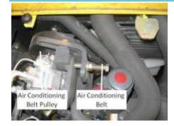
**Details** Air conditioner compressor belt pulley and air conditioner compressor belt.
