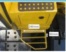
**Details** Dimensions of openings in Step 1 floor on right hand side (i.e. maintenance) access system are 240 mm x 50 mm.
