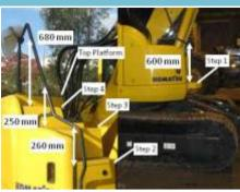
Vertical distance between step 1 nosing and the handrail on the right hand side (i.e. maintenance) access system is 600 mm. Vertical distance between step 2 nosing and the handrail on the right hand side (i.e. maintenance) access system is 260 mm. Vertical distance between step 3 nosing and the handrail on the right hand side (i.e. maintenance) access system is 250 mm. Vertical distance between step 4 nosing and the handrail on the right hand side (i.e. maintenance) access system is 680 mm.
