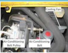
**Details** Cooling fan & air conditioning belt guarding.
