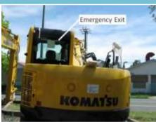
**Details** Emergency egress located near engine compartment.
