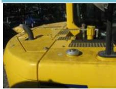
**Details** Top platform of machine has no guard railing.
