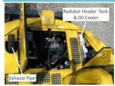
**Details** Exhaust pipe, radiator header tank and oil cooler.
