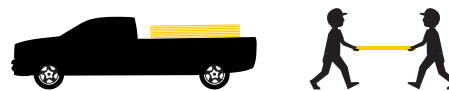
ROADPLATE Transported by Ute or small truck and positioned by two men
