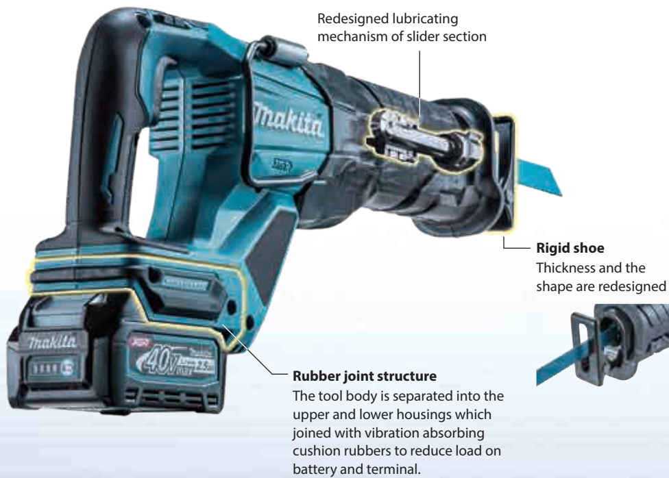
Smooth cutting with vertical crank system
