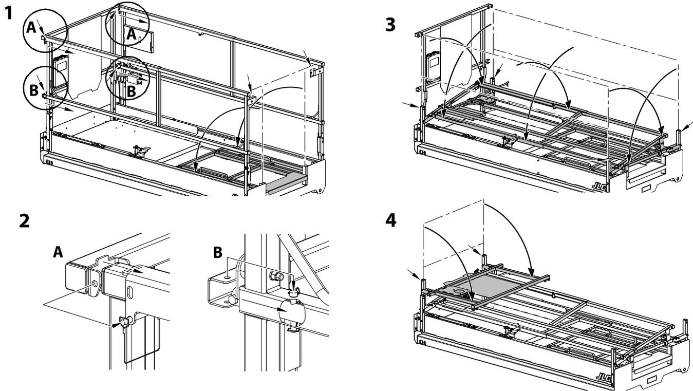
Figure 3-2. Platform with Rail in Rail Extension - Fold Down Sequence
