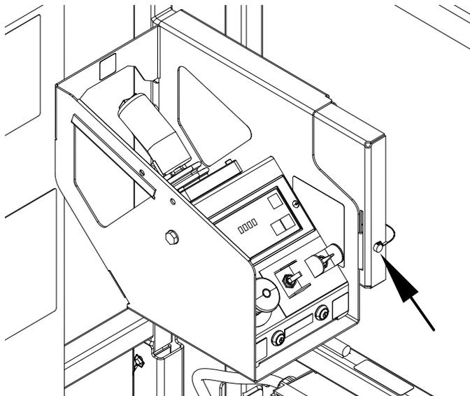
To prevent unauthorized removal, the platform control station can be secured to its mount by replacing the lock pin located on it's mounting tab with a keyed or combination lock.
