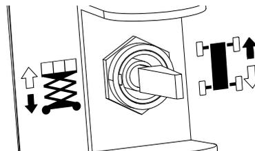
This toggle switch is used to select operation of either the drive or lift function. After selecting a function, the joystick controller must be used in order to activate that function. Only change the function selected, with the joystick in the neutral position. Otherwise, the function selected will not change until the joystick is returned to the neutral position.
