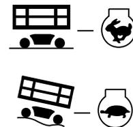
**NOTE:** Drive speed will automatically be reduced to low drive when the platform is raised above the stowed position, regardless of speed switch position.
