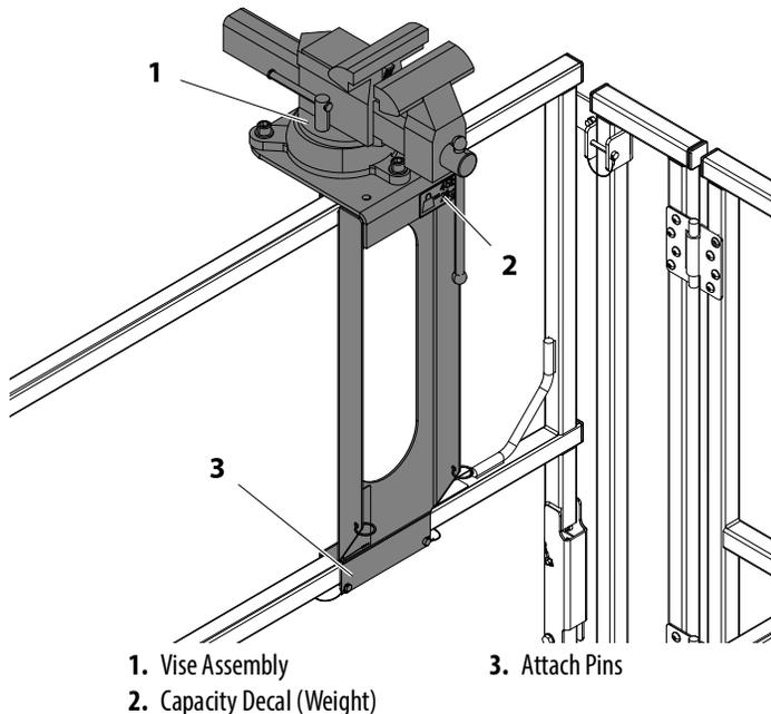
**NOTE:** If the WorkStation is installed, it must be mounted to the opposite side of the platform from the Vise.
