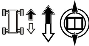
The drive system is proportional: for additional drive speed, push the joystick further from the neutral position in the direction of travel. Releasing the trigger switch or returning the joystick to center will stop machine movement.
