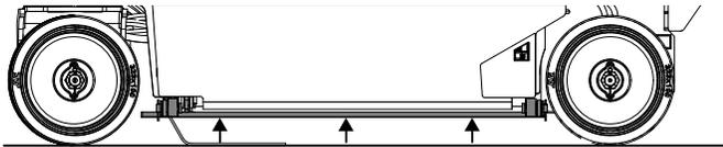
Platform Fully Lowered - Pothole Bars Raised
