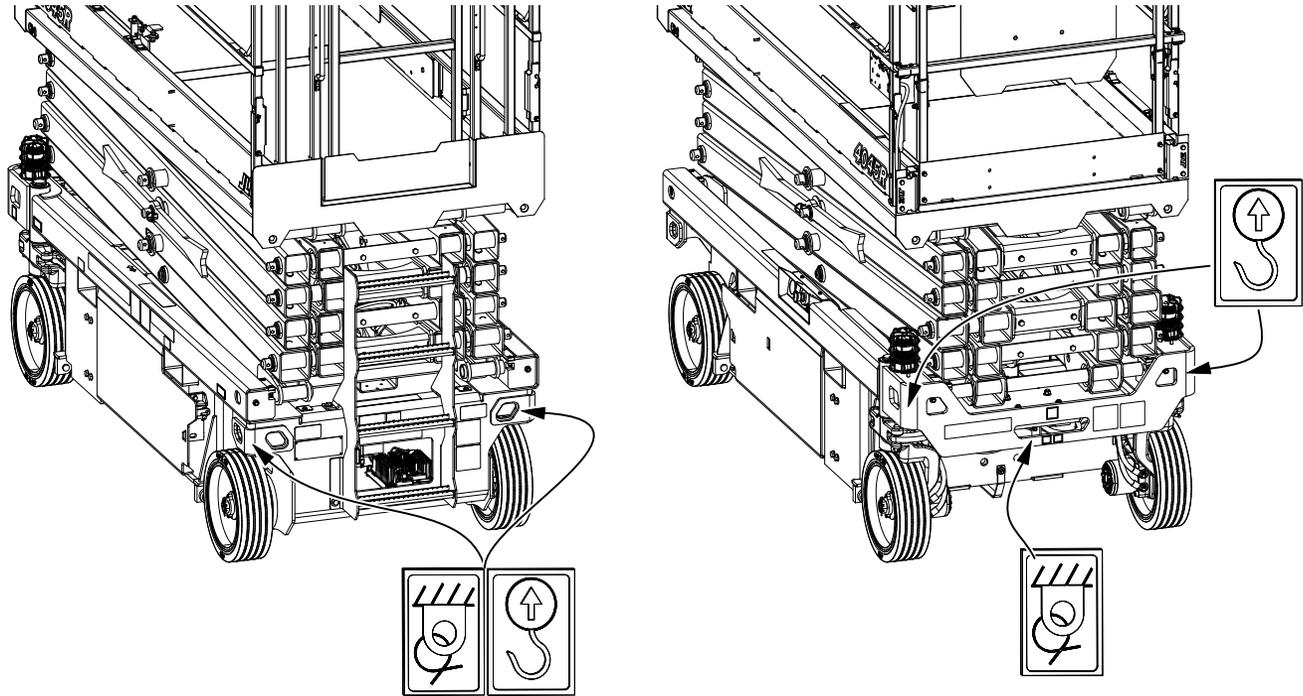
Figure 3-5. Tie Down and Lift Lug Locations
