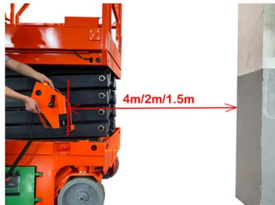
Ultrasonic safety sensor
