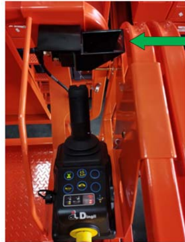
Ultrasonic safety sensor
