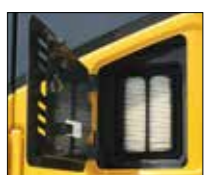
External air conditioner filter
