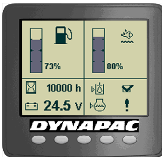
Fig. Status screen with "DailyCheck"
