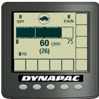
Fig. Compaction meter display (CMV display)
